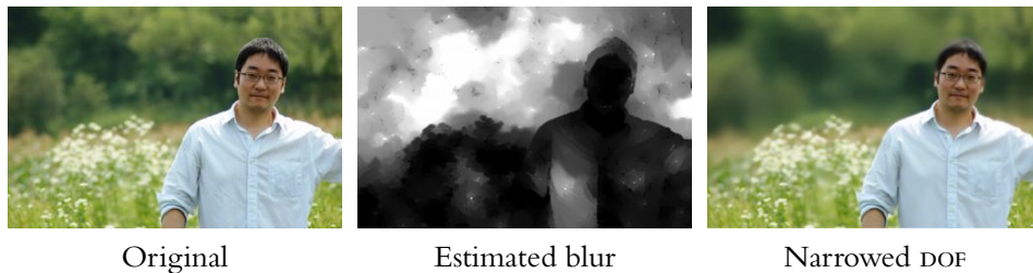
Figure 3.11: Example of input image (left), estimated blur map (center) and Bae and Durand [2007] blur magnification (right). Images copyright Soomin Bae.
