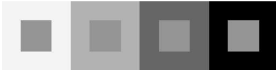
Figure 2.14: Example of simultaneous contrast. The internal gray squares appear of different brightness depending on the surrounding area.
