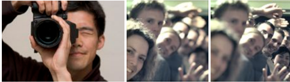
Figure 3.1: Plenoptic camera of Ng et al. [2005] (left). The combination of microlenses and processing allow the image to be refocused after capture Images copyright Ren Ng.
